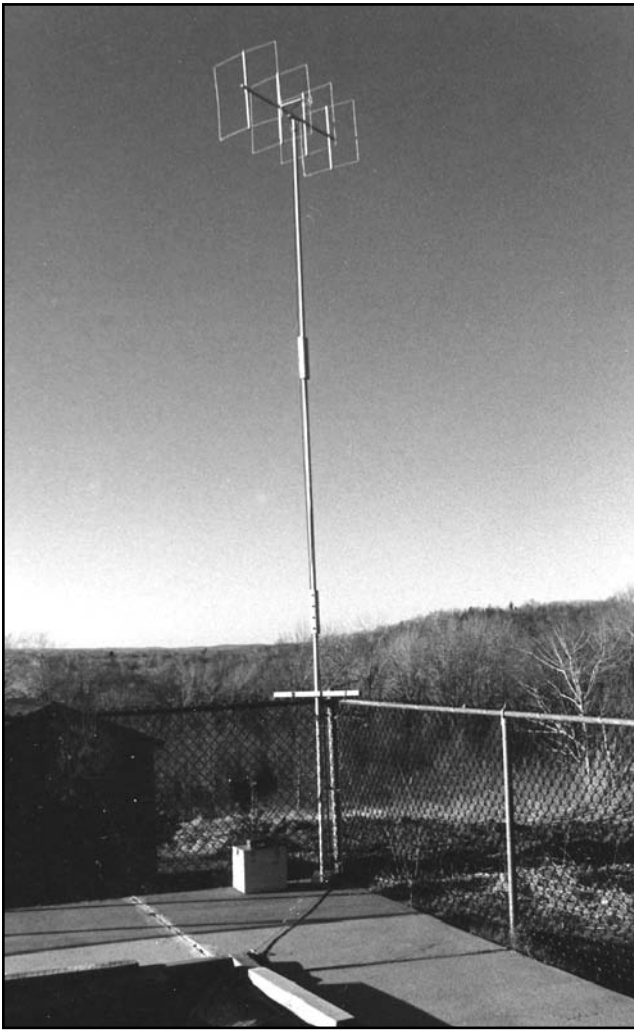
Fig 56 —The 4-element 144-MHz portable quad, assembled and ready for operation. Sections of clothes closet poles joined with pine strips make up the mast. (Photo by Adwin Rusczek, W1MPO)
